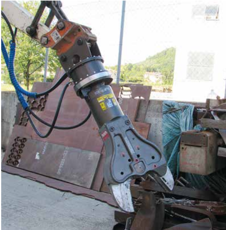
CESOIA F200C CON LAME AD INSERTI INTERCAMBIABILI CUTTER F200C WITH REPLACEABLE CUTTING EDGES COD. 1.50.2380
